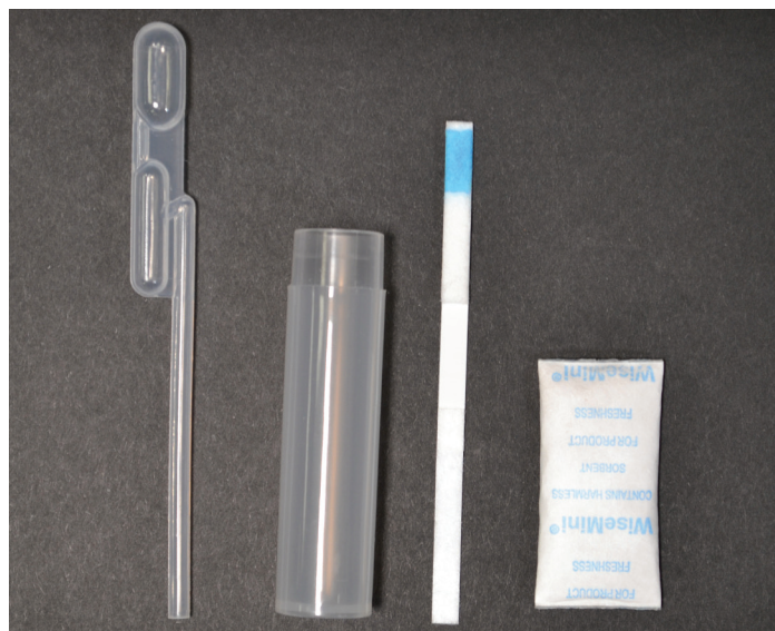
Test kit components (from left to right): volumetric pipette, test vial, test strip, desiccant
