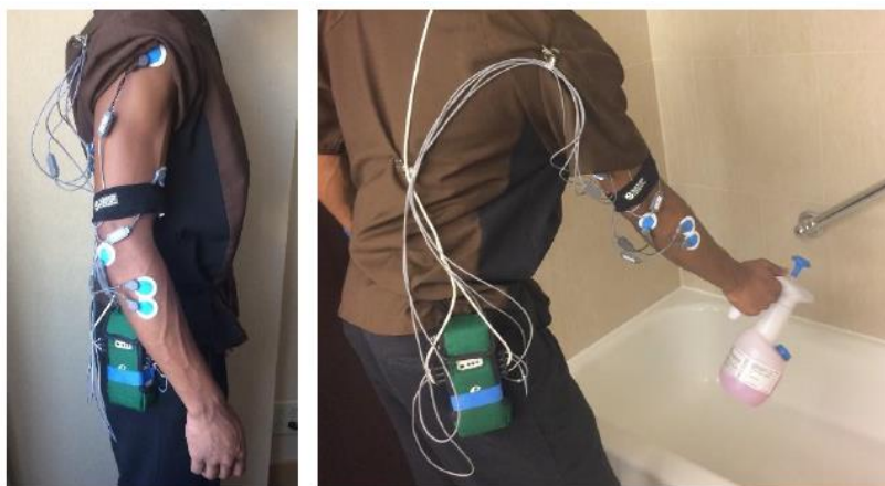
Illustration of test participant wired for electromyography
