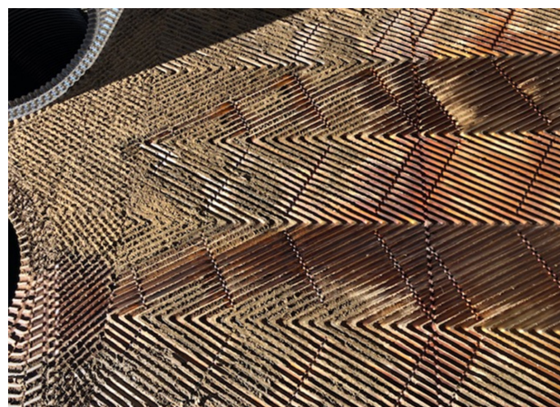
Figure 2. Plate from a heat exchanger taken apart during an ammonia production downturn. The grooves on the top of the plate are covered with a biofilm, adding a layer of thermal insulation.
