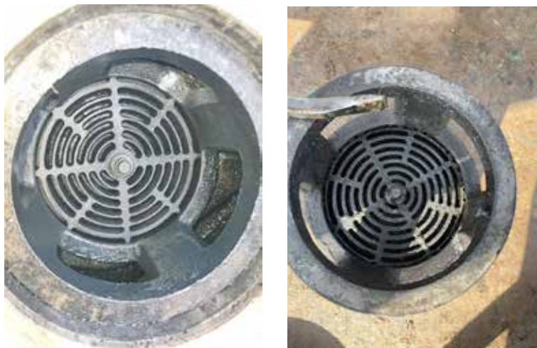
Figure 2. Compressor valve two weeks into the trial (left) and after the 10-week trial (right).
