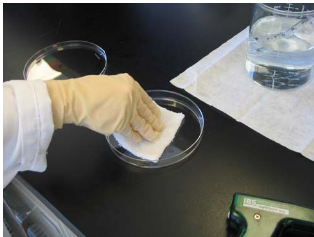
Figure #4: Cotton cloth swatch saturated with product B applied to a contaminated petri plate.
