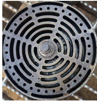
Figure 2: Compressor valve after Inlet Integrity Program implementation.
