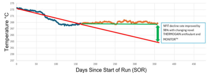
FIGURE 2: NFIT data recorded prior to and following the implementation of the THERMOGAIN antifoulant trial
