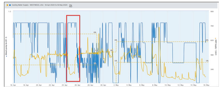
FIGURE 4: On 24-25 April, oxidation-reduction potential (ORP) declined, but the bleach pump relay indicated the pump was running. However, the bleach pump had failed. Once the pump was repaired, ORP increased and the deposit risk index declined, indicating a clean-up of the biofilm.
