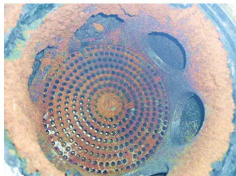
FIGURE 1: A typical compressor valve with fouling.
