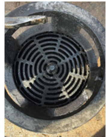
FIGURE 4: Compressor #7 valve after ten weeks of chemical feed.
