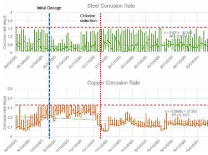
Figure 3. Steel and copper corrosion rate as read by the Nalco Corrosion Monitor
