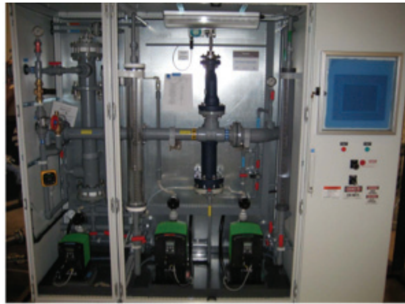
Figure 1 -PURATE SVP Pure chlorine dioxide generator (SVP-Pure ClO 2 Generator (MSA)).
